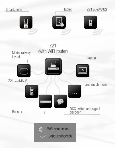
The Z21 system is compatible with many well-established PC-based model railway controllers. Furthermore the system is perfectly suited to control your garden railway.
