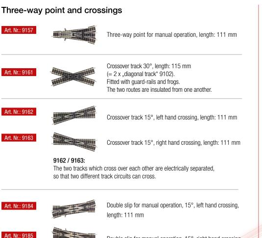
Double slip for manual operation, 15°, right hand crossing, length: 111 mm
